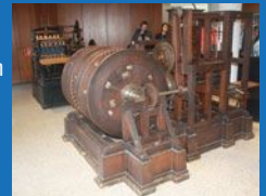
An early Koenig & Bauer printing press made of wood
